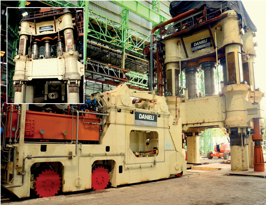
The newly installed 6000 T Forge Press under the final stages of commissioning
