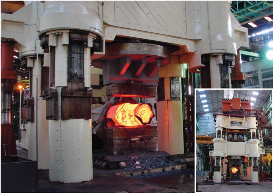
The newly commissioned 6000 T Forge Press
