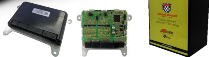
Battery and BMS
