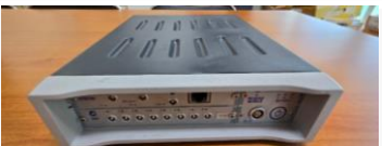
Siemens SCADAS Mobile (Acoustic test machine)
