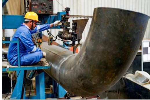
Automatic GMAW Welding System
