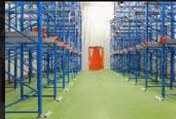
DRIVE-IN PALLET RACKING
