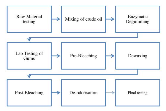
**Raw material testing**: Upon receipt of the raw materials, our Quality Division tests the crude oil to assess its physical composition as per the parameters defined.. The quality of the oil is also checked to ensure that our final products meet with the quality requirements of our customers and regulatory agencies.
