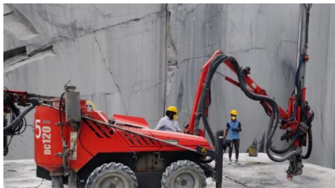
Drill machine equipped with dust sucking mechanism
