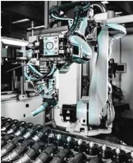
▲ Exhaust Gas Recirculation pipe assembling on Medium Diesel Engine exhaust manifold in the plant at Lombardore, Italy
