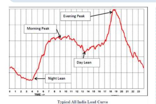
As it can be seen from a typical load curve in India, peak demand is post 5pm which supports our argument that coal based power is integral to cater to base load till affordable storage comes in a major scale.
