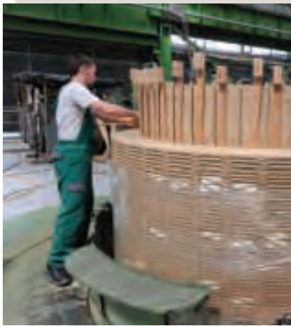
Coil Winding process undertaken at CG Hungary transformer factory, which is a pioneer for 765 kV technology
