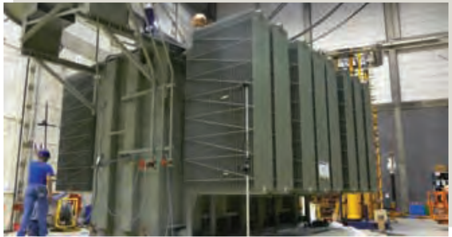
CG Power now manufactures transformers that produce 40 dBA sound pressure at 30cm, that is no more than the sound of a humming mosquito
