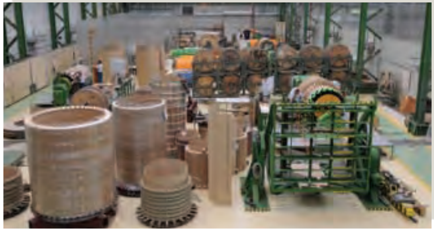
Coil Winding process undertaken at CG Hungary transformer factory, which is a pioneer for 765 kV technology
