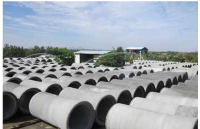
1900 mm dia PSC Pipes manufactured at Chilamathur Factory for Pulakurthy Lift Irrigation Scheme, Andhra Pradesh
