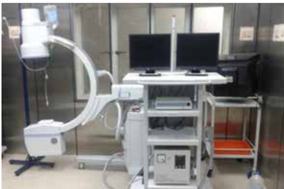
Allengers HF-49R/PS100 High Frequency (40 KHZ) Mobile C-ARM Machine with accessories used in Orthopedic Department in Government Royapettah Hospital, Chennai, Tamilnadu
