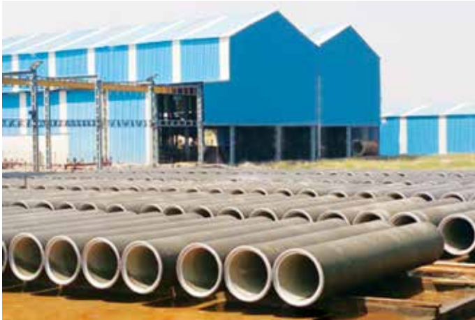
1000 mm dia PCC pipe manufactured at Dhule factory for Jalgaon Jamod Water Supply Scheme, Maharashtra
