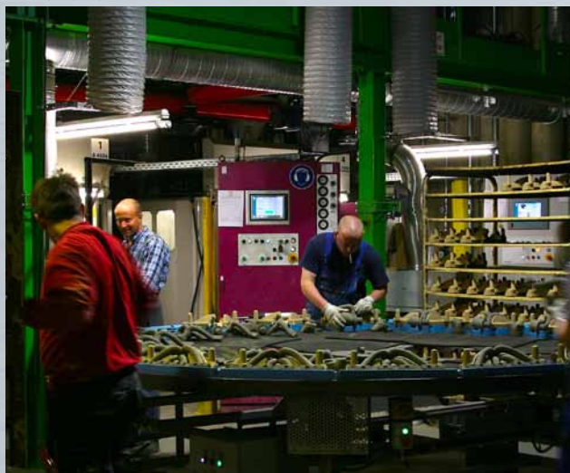
Assembly of core packages at the core shop at Eisenwerk Erla GmbH, Germany, which are used for the castings of Integrated Turbine Housings produced for Audi AG through IHI Charging System.
