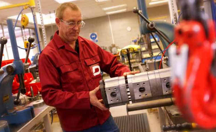
Assembly of the new Triple Pump from the John Deere Thor series at Dynamatic's Hydraulic Facility at Swindon. Dynamatic®, Swindon, commenced supplies of the Thor range of pumps to John Deere, Waterloo, in November 2011.
