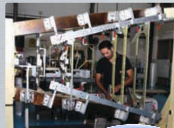
JIG Assembly for Bell 407 at Dynamatic Park, Bangalore
