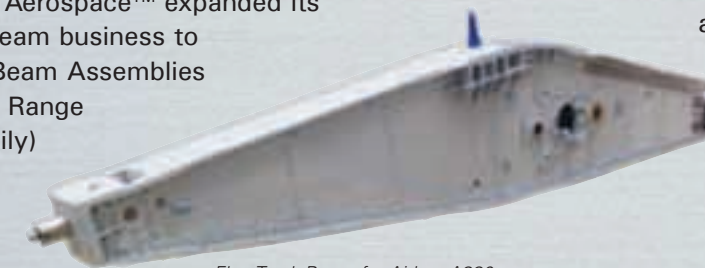
Flap Track Beam for Airbus A330 Assembly scheduled to commence in 2015 at Bangalore
