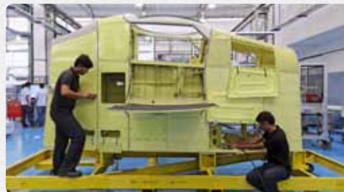
Aft Pylon Assembly and Cargo Ramp Assembly for the Boeing Chinook CH-47F Helicopter at Dynamic Park, Bangalore
