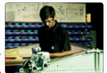
Assembly of Flap-Track-Beams for Airbus A320 Single Aisle Aircraft at Dynamatic-Oldland, Bangalore, India
