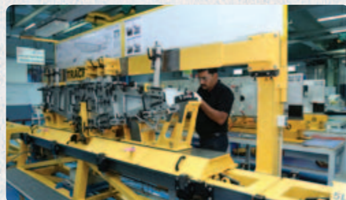
Stage 1 Assembly line for Airbus A330 Flap-Track-Beams (above)
