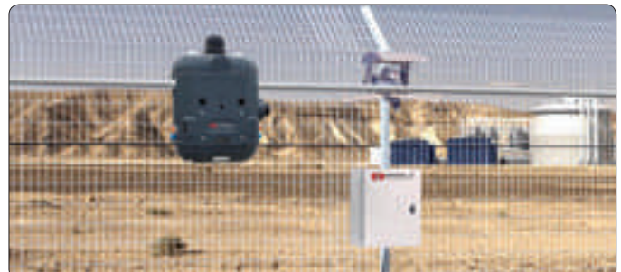
RoboGuard is a revolutionary agile scout robot, which runs along secured fences, ensuring perimeter integrity and capable of responding promptly to intrusion alerts. It consists of an autonomous unit, travelling on a monorail and carrying several sensors. (photo credits: magal)
