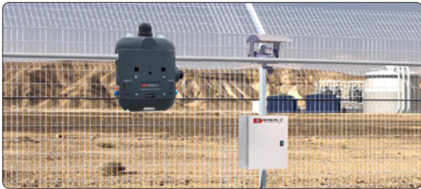
RoboGuard, a product by Magal - Israel, is a revolutionary agile scout robot, which runs along secured fences, ensuring perimeter integrity and capable of responding promptly to intrusion alerts. It consists of an autonomous unit, travelling on a monorail and carrying several sensors. (photo credits: Magal)
