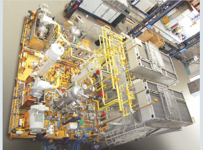
LP Gas Compressor Package for ONGC (MHN) offshore platform
