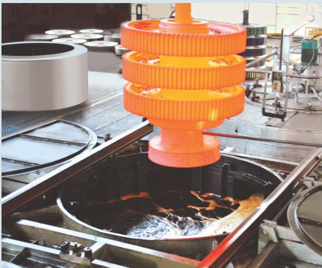
Gears during Heat treatment
