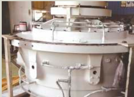
1 MW Planetary Gearbox for Windmills.
