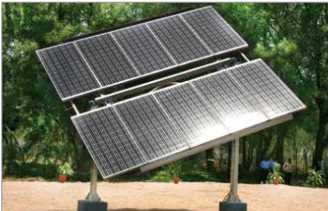
Indigenously developed Solar Thermal Sun Tracker based on Liquid Balancing System
