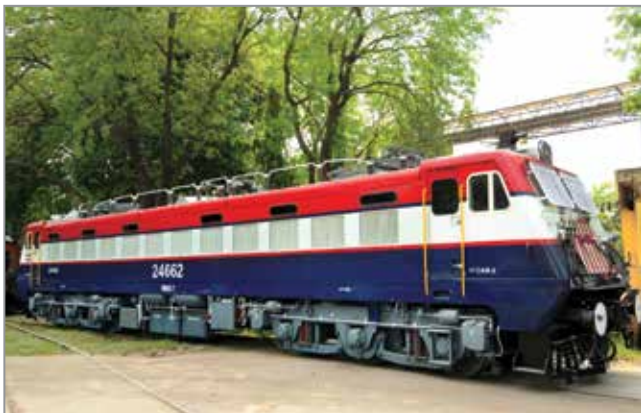
Electric Locomotive (25 kV AC, Type WAG 7)
