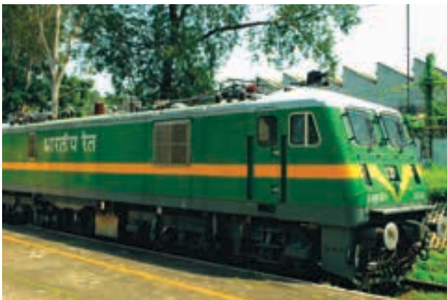
WAG-9 locomotive with IGBT based three phase drive propulsion system
