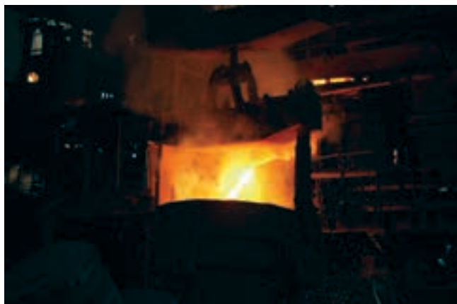
Recycling of MS scrap for producing molten steel required for steel forgings & castings at Steel Melting Shop, CFFP, Haridwar
