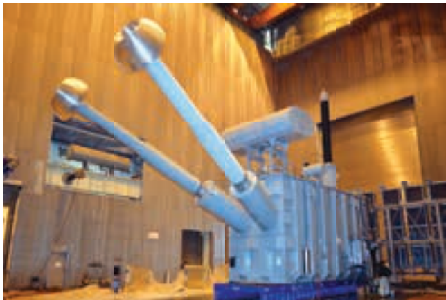
400 kV Class HVDC Converter Transformer under test at BHEL, Bhopal for \pm 800 kV, 6000 MW, multi-terminal HVDC NE Agra project
