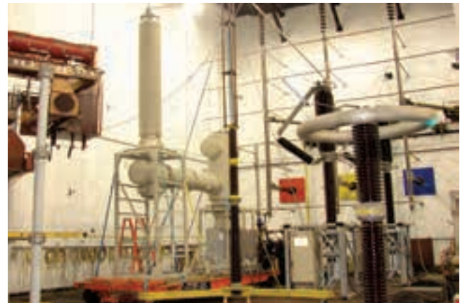
420 kV, 40 kA, Single Break GIS Circuit Breaker using spring hydro drive developed and tested successfully by BHEL
