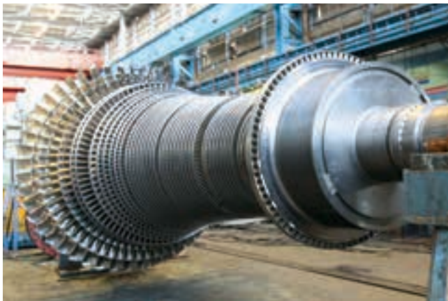
New variant of single cylinder reheat turbine of 125 MW rating with improved efficiency developed by BHEL
