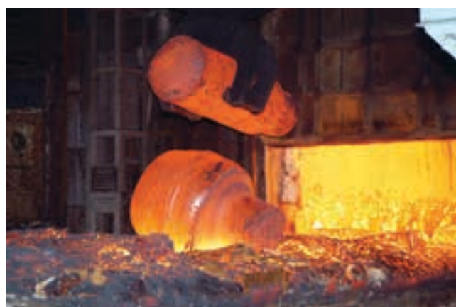
Diesel Oil operated furnaces converted to Natural Gas at CFFP, Haridwar to reduce emission of greenhouse gases
