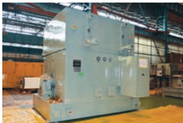
20.5 MW 11 kV 4 POLE, 1500 RPM Motor developed for Boiler Feed Pump application
