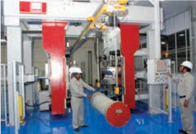
State-of-the-art facility for manufacturing composite hollow insulators up to 800 kV rating, developed by BHEL
