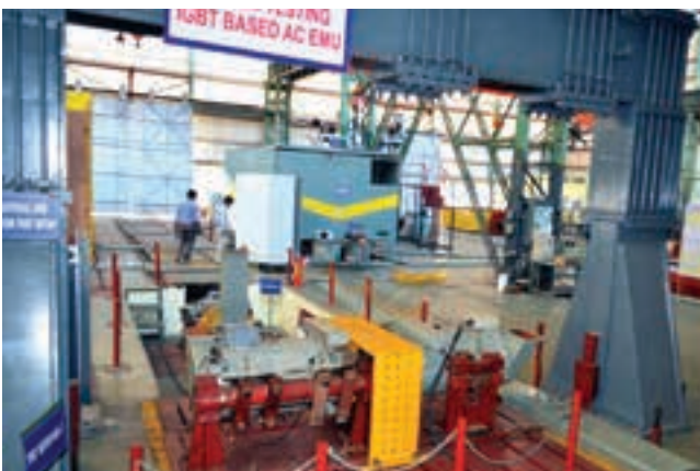
Integrated testing of the traction platform for the state-of-the-art IGBT based propulsion systems for AC EMUs at EDN, Bangalore
