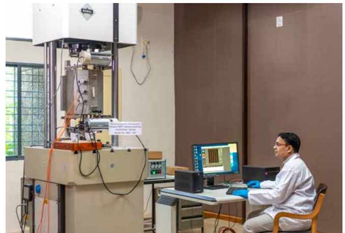
Ambient and high temperature tensile and Low Cycle Fatigue (LCF) test facility for metallic materials at Corp. R&D, BHEL Hyderabad
