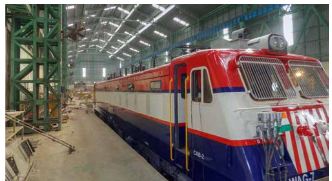
WAG 7 5000 HP locomotive with regenerative braking system under final stages of production at BHEL, Jhansi
