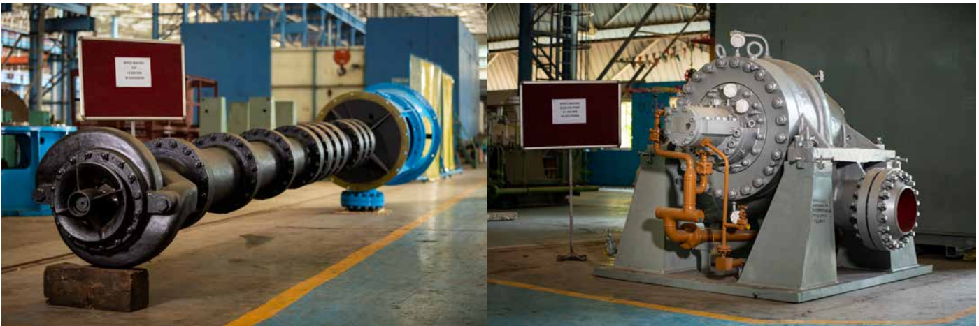
BHEL manufactured Condensate Extraction Pump (left) and Booster Pump (Right) ready for dispatch for BIFPCL Maitree project, Bangladesh
