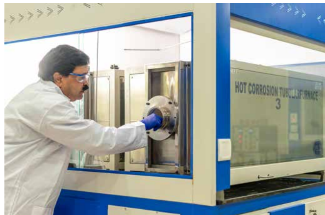
Furnaces for testing fire side corrosion of alloys and welds at Corp. R&D, Hyderabad
