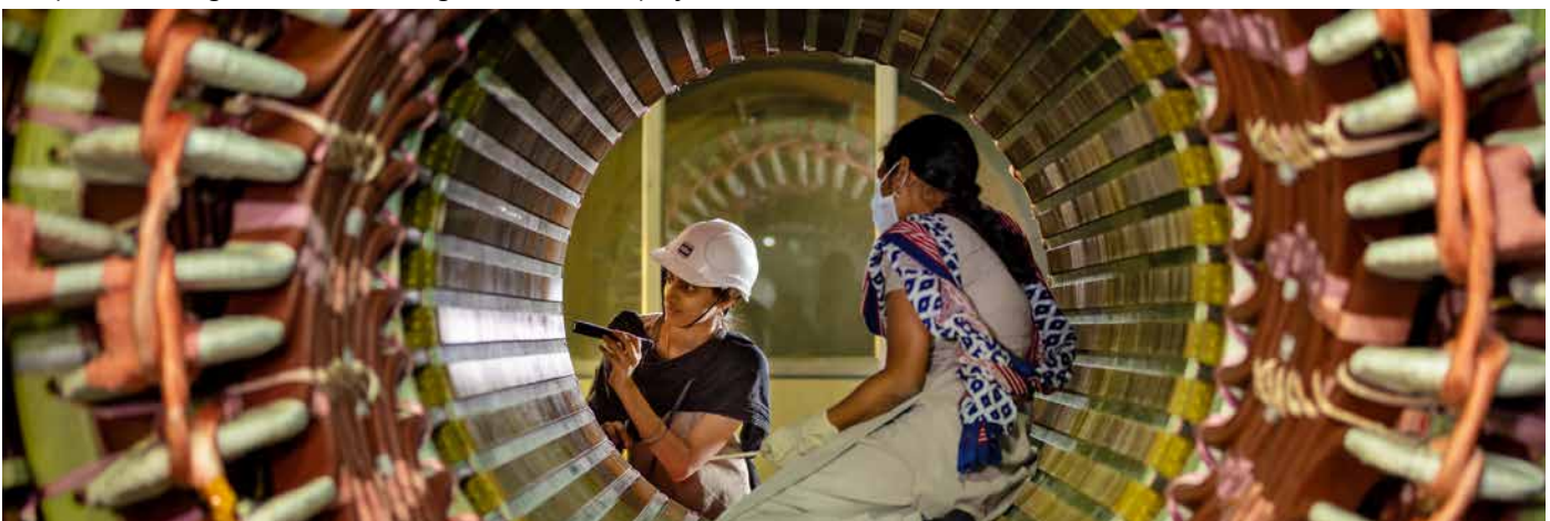
Engineers inspecting the assembly of generator stator in HPEP, Hyderabad
