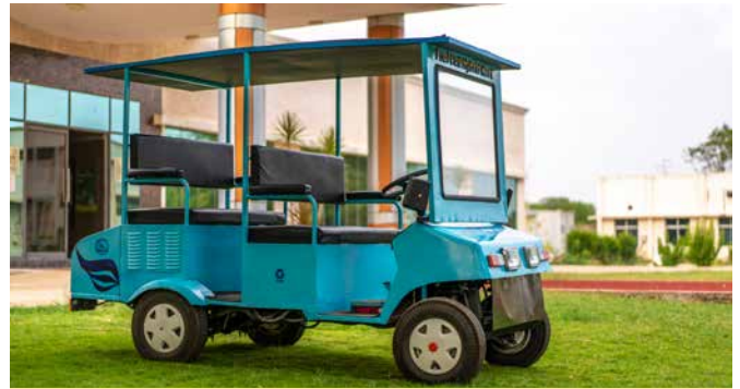
Fuel cell powered 1.25 kW hybrid electric golf cart vehicle developed by BHEL
