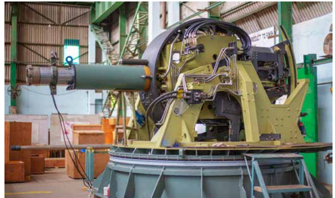
Super Rapid Gun Mount (SRGM), for Indian Navy being manufactured at BHEL Haridwar plant
