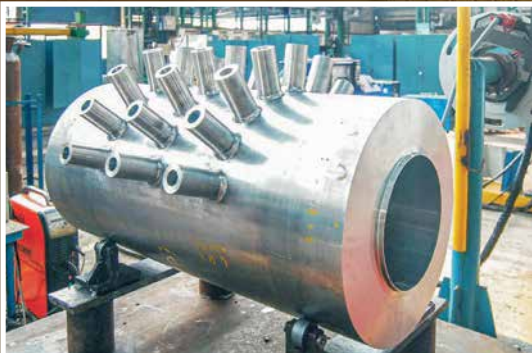
Mock-up thick-walled superheater header for AUSC boilers with advance high temperature materials
