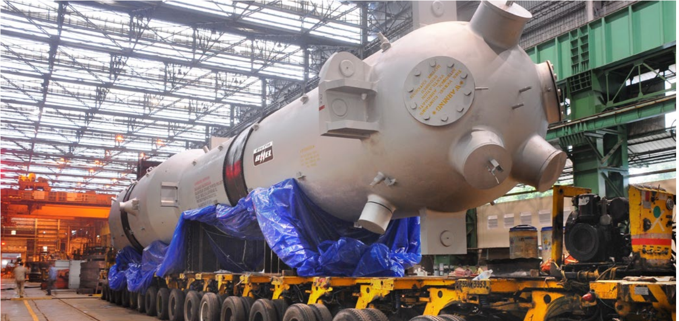
BHEL dispatched its 40 th Nuclear Steam Generator to NPCIL for installation at Rawatbhata Atomic Power Project
