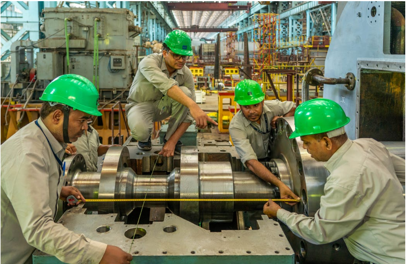
Steam turbine rotor shaft under inspection at HEEP, Haridwar
