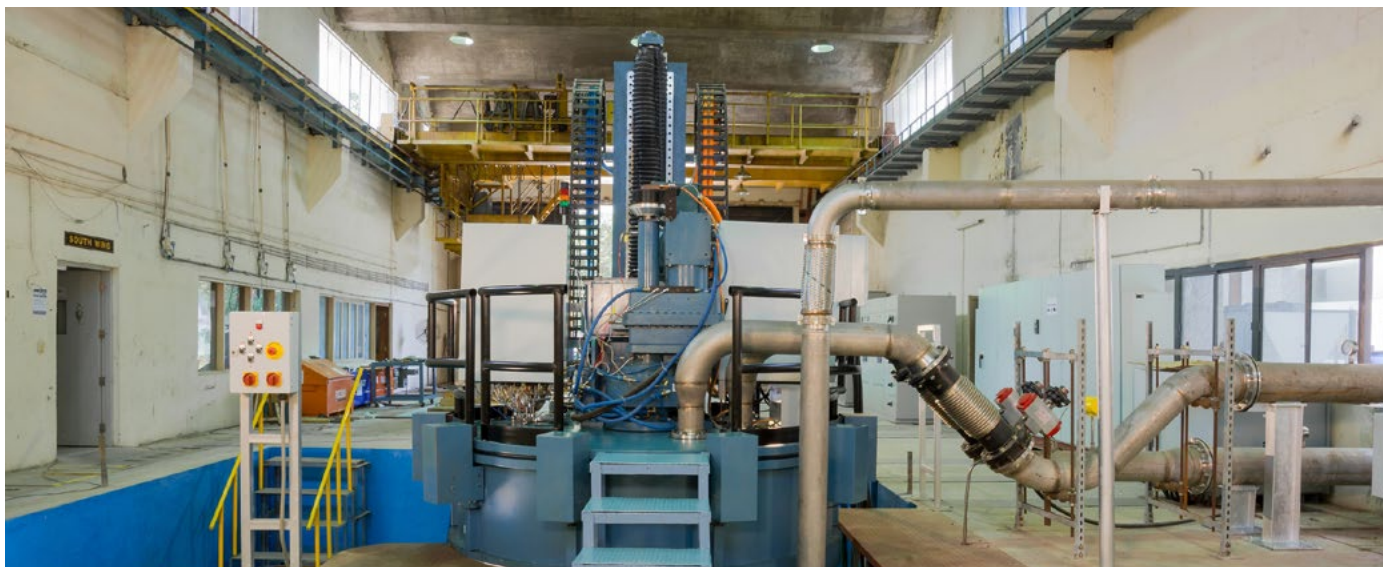
Unique High Temperature Spin Test Rig (HTSTR) established for testing of advanced materials for AUSC mission project
