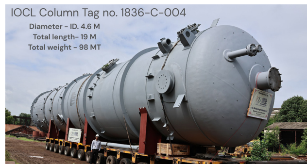
Pressure Vessel Column supplied to IOCL, Vadodara Refinery
